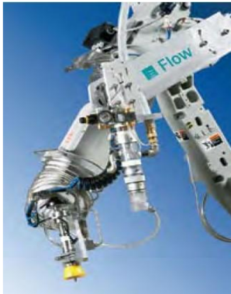
Fig. 8 – Robot in 6 axes of processing with water jet (Herghelegiu, 2011; flowcorp.com).
